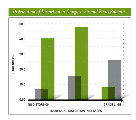
Douglas-fir is highly regarded for its stability, meaning that it stays straight. There are very few issues with longitudinal shrinkage near the pith, spiral grain and compression wood' and as a result its shape is retained when dry. Its steady nature and strong character help prevent movement in building structure and ensures a cleaner finish for interior linings.
